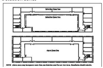
In order to give a clear indication of fire location, buildings are split into detection zones. Zones containing just call points are usually restricted to a maximum floor area of 2000m2.
