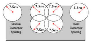
This depends on ceiling height, pitch and structure. For flat ceilings no point on the ceiling should be more than 7.5m from the nearest smoke detector (5.3m for heat detectors). In corridors less than 2m wide only the centre line need be considered i.e. smoke detectors would be placed 7.5m from the end walls and then at 15m intervals.
