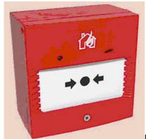
Manual call points need to be prominently sited and distributed so that they can be readily observed by persons leaving a building. Normally the evacuation signal should be sounded within 3 seconds of actuation.
